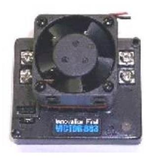
• The high current capacity, low voltage drop, and peak surge capacity make the Victor 883/4 ideal for drive system, while its breaking option and precise control meet the demanding needs of arms and lift systems.
